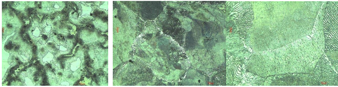
Fig.1 Microstructure of LAZ661 alloy (a) as-cast, 200X (b) Homogenized at 450 0 C-12h, 200X (c) Homogenized at 450 0 C-12h, 500X
