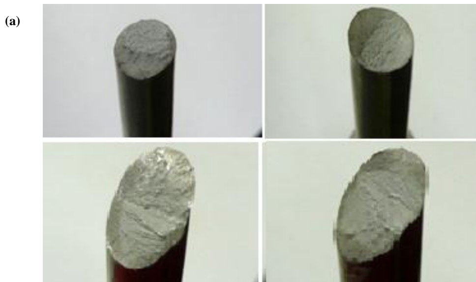
Fig.9a Cup cone fracture and shear fracture after tensile test.
