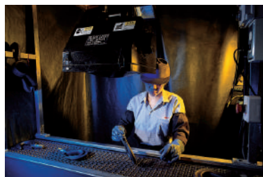
Magnaflux Crack Detection
