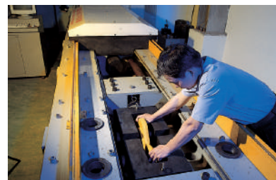
Tensile Test, Capacity 300 tons
